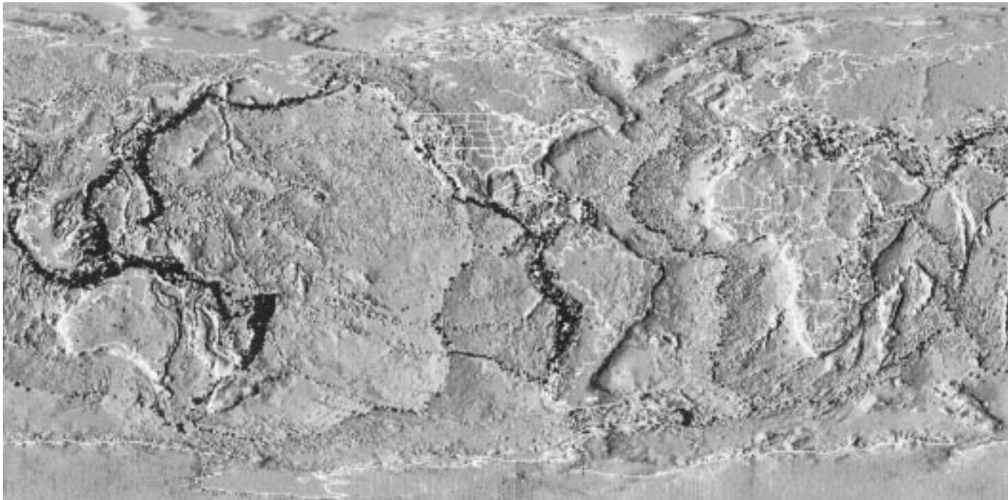
FIGURE 5.2: Global seismicity and major tectonic plate boundaries.
